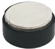
Fig. 1. GelTac prototype with 3d-printed shell and camera case, silicone lens hood and rubber-like elastomer cover
